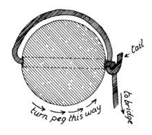
STYLIZED CROSS-SECTION VIEW OF FRICTION PEG AND STRING WINDING —NOTE HOW THE WINDING BINDS ON TOP OF THE SMALL PIECE OF STRING TO KEEP THE STRING FROM COMING LOOSE
